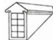
Dormer A roofed structure containing a window.
