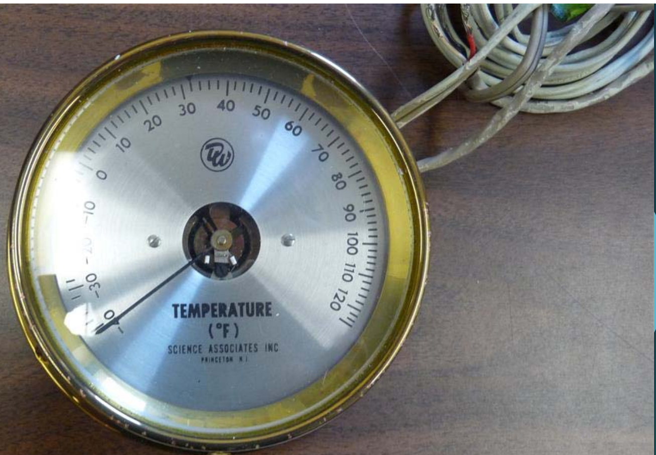
TEMPERATURE INDICATOR Science Associates, Inc.
