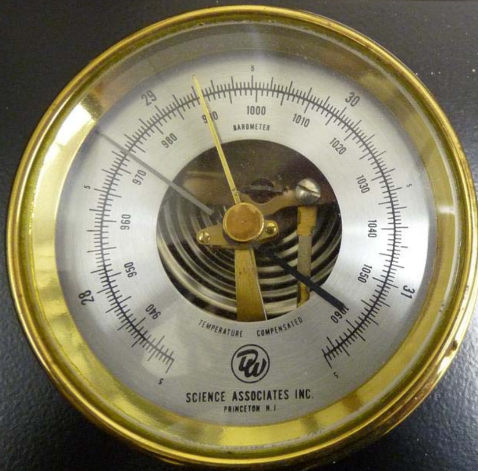
ANEROID BAROMETER Science Associates, Inc.
