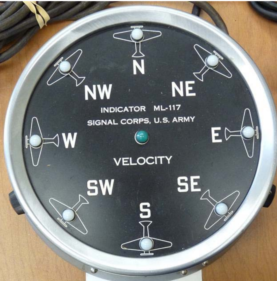
WIND INDICATOR U.S. Army Signal Corps
