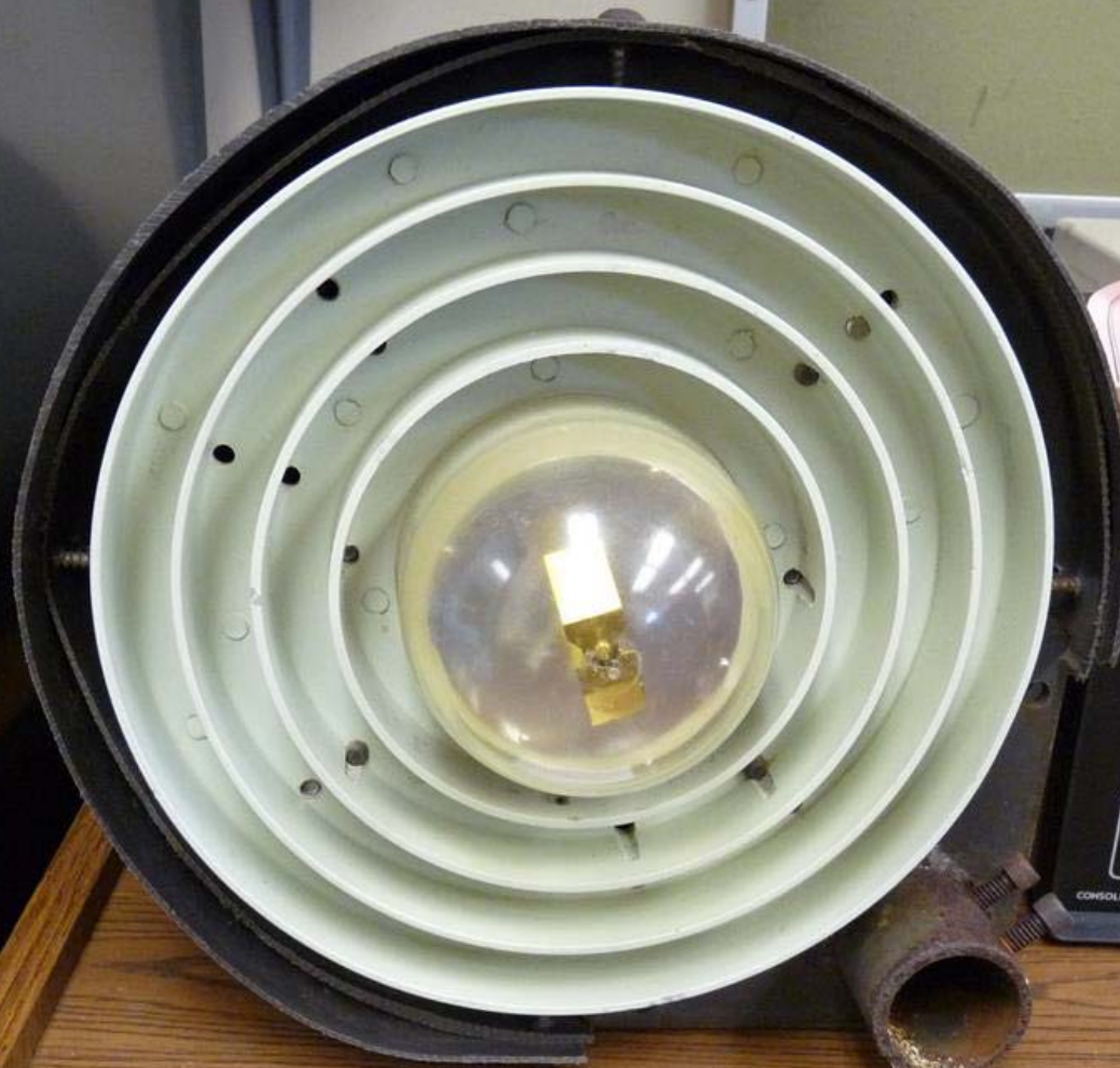
SATELLITE ANTENNA HORN
