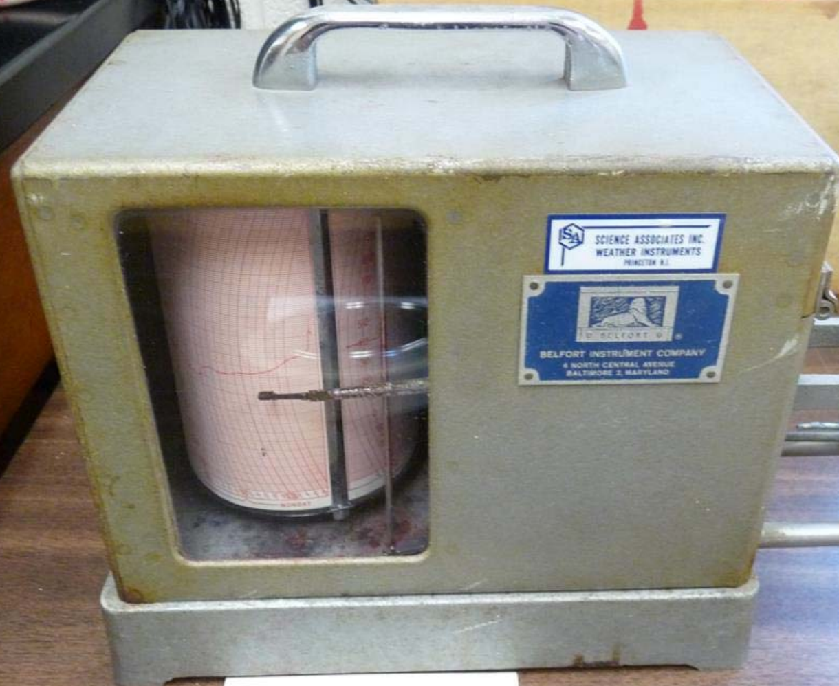
THERMOGRAPH Belfort Instrument Co. Baltimore, MD
