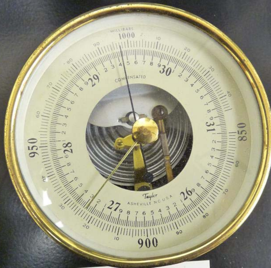
ANEROID BAROMETER Taylor Instruments
