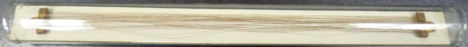
HYGROMETER Hair-Fiber Sensor
